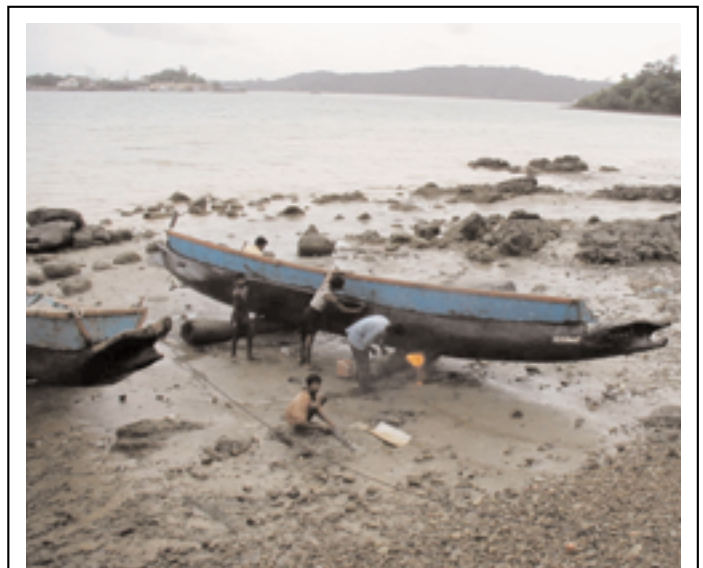
Figure 3 Tarring the bottom of a traditional mechanised craft or Dhonghi in Panighat.
