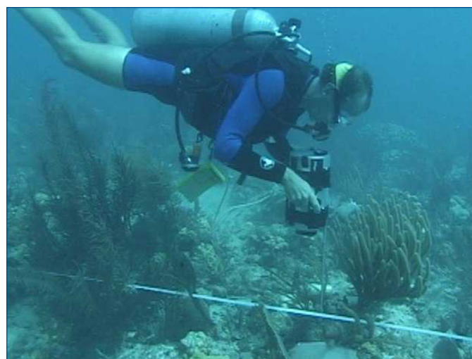
Diver using a sonar positioning system and video camera to record transect data in the U.S. Virgin Islands
