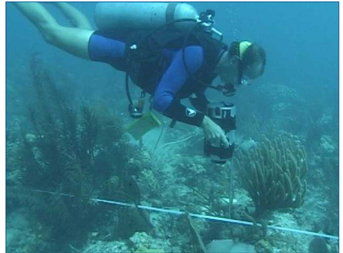
Diver using a sonar positioning system and video camera to record transect data in the U.S. Virgin Islands
